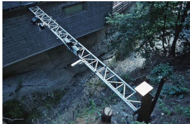
Figure 5. Video and flow depth monitoring station Pians (lower reach).
